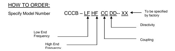
**Example:** To order a WR42 18 to 26.5 GHz Waveguide Crossguide Block Coupler with frequency band of 18 to 26.5 GHz, 20dB coupling level, a 15dB directivity, specify CCCB18262015-XX.
